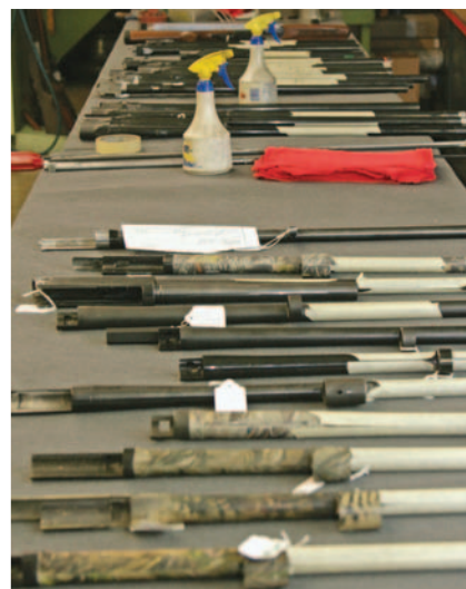
THESE BARRELS AWAIT THEIR TURN ON THE EDM MACHINES. DEMAND FOR PORTING REMAINS STEADY AND WHEN MIXED WITH THE PISTOL WORK AND RIFLE BRAKES, KEEPS THE STAFF HOPPING.
