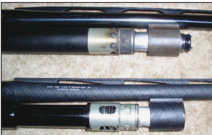
TOP: GAS VALVE IN THE GOLD AND SILVER SPORTING. BOTTOM: NEW MAXUS VALVE.
