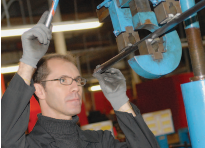
THE TRUENESS OF THE BARRELS IS STILL CHECKED BY EYE.
