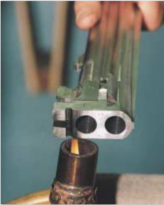
ALL PARTS ARE FITTED TO 'A THICKNESS OF SMOKE' TOLERANCE.
