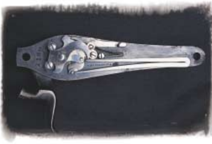
ABOVE: A TYPICAL BACK ACTION SIDELOCK OF THE TYPE COMMON ON BREECHLOADING HAMMER GUNS OF THE 19TH CENTURY. NOTE THE MAINSPRING TO THE REAR OF THE LOCK. ...
