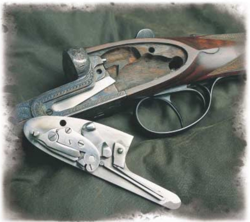
BELOW: ...CONTRAST THIS WITH THE BAR ACTION LOCK FOUND ON VIRTUALLY ALL HAMMERLESS SIDELOCKS. THE SPRING IN THIS CASE LIES TO THE FRONT IN THE ACTION 'BAR'.
