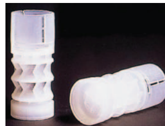
A TYPICAL EUROPEAN 12 GAUGE INTERNATIONAL TARGET WAD (B&P) DESIGNED FOR 24 GM OF SHOT IN THE 2\frac{3}{4} INCH HULL. \frac{3}{4} OZ OF SHOT GENERALLY FILLS THE CUP OF THESE WADS TO THE TOP OF THE PETALS OR SLIGHTLY HIGHER, AND WORKS GREAT WITH STANDARD 24GM INTERNATIONAL TARGET LOAD DATA IN 2\frac{3}{8} INCH (67MM) HULLS, WITHOUT THE NEED FOR CARD INSERTS IN THE SHOT CUP.
