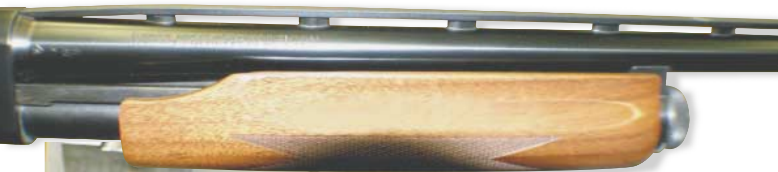
A COMPLETED RIB JOB ON AN OLD REMINGTON 870 THAT WAS ORIGINALLY A PLAIN BARRELED GUN.
