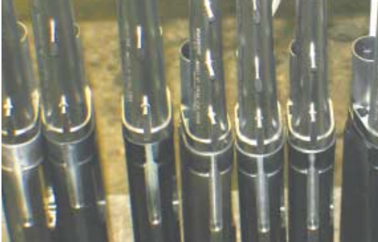
A DOZEN WINCHESTER MODEL 12s WITH POSTS IN PLACE, WAIT FOR THE RIBS TO BE INSTALLED AND THEN BLUED.
