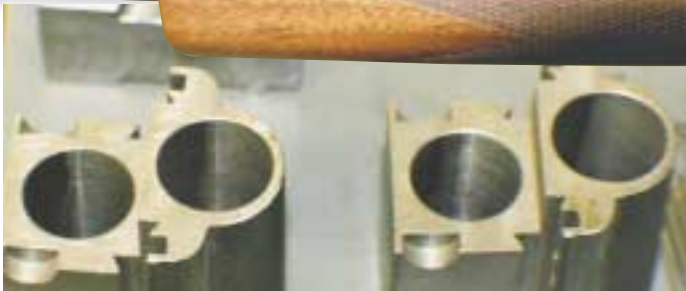
RAW MONOBLOC'S READY TO BE MACHINED AND FITTED UP WITH EXTRACTORS AND BARRELS.
