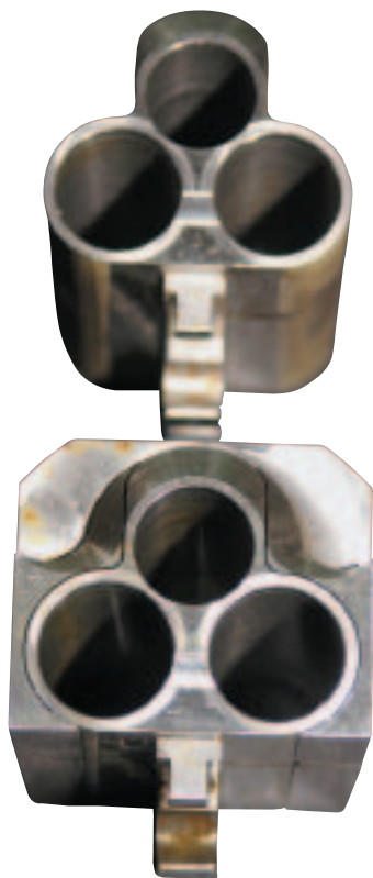
THE PRECISION OF EDM MACHINING IS SHOWN BY THIS BEFORE AND AFTER SHOT OF THE MONOBLOC FOR A 'DRILLING' COMBINATION RIFLE/SHOTGUN.
