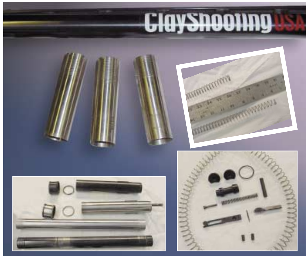
MAIN PICTURE: THIN WALLED CHOKES CAN BE INSTALLED. INSET LEFT: FACTORY BLUED GAS SYSTEM CAN BE HARD CHROME PLATED (MIDDLE PARTS) TO INCREASE LONGEVITY AND TO MAKE CLEANING EASIER. INSET TOP: RECOIL SPRING (TOP) READY FOR REPLACEMENT. INSET BOTTOM RIGHT: SOME SUGGESTED SPARE PARTS.
