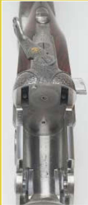
THIS VIEW CLEARLY SHOWS THE KERSTEN CROSS BOLT OF THE BERETTA SO.
